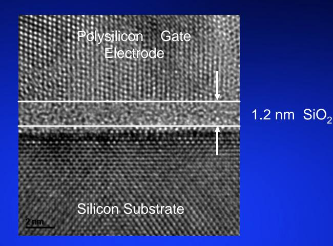
Gate oxide is less than 5 atomic layers thick
